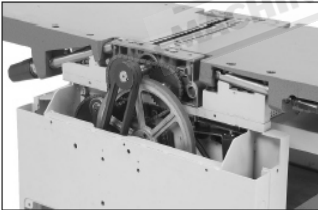
Figure 46. Fence and V-belt cover removed.
